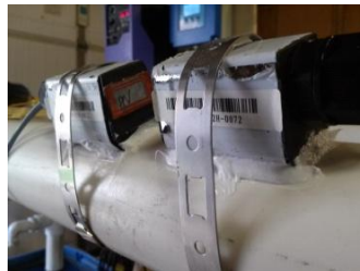
Band Mounting Transducers (2" - 30" Pipes)
