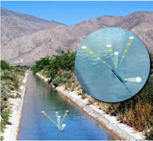
Actual picture of open channel acoustic discharge Doppler meter with close-up graphic depicting operation
